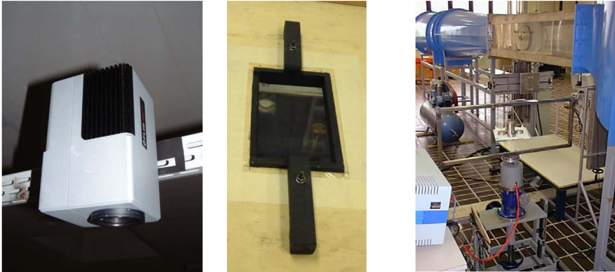
Fig. 3. The IR thermographic camera (a) , the IR window (b) and the 6 axis Load Balance (c).
