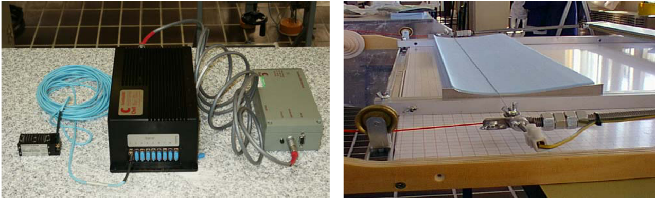
Fig. 5. The Multipressure Scan System (a) and the Airfoil Section cutting machine (b).
